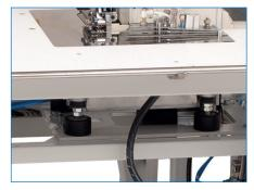
The sewing unit FX 2300-EXT is the economy version for sewing sideseams and inseams. The compact design is especially suitable for the universal use in the production of sportswear trousers. Due to the pneumatically moveable edge guide it is possible to trim the excess lengths of pocket bags.
