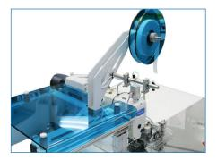
GG 5100 Tapes can be attached to jacket Chest Canvas. With a low work input this automatic unit guarantees high quality combined with high efficiency. The machine is equipped with a tape feeding device, tape cutter, thread trimmer and the option to predetermine the seam length. The tape feeding device guarantees reliable tape feeding.
