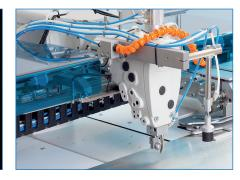
JX 5300-IX is designed for consistent and productive Top Stitching on the Left Trousers Fly of formal and casual trousers with one or two parallel seams. Thus, this sewing unit is not only suitable for the production of classic trousers but also for the production of Dockers, Chinos etc. On any sewing style the operator positions the front trousers with the help of a laser marking. The seam-end is precisely in the seam shadow of the lower waistband edge or optionally at the upper waistband edge.
