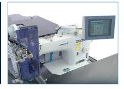
XP 7100 - IX Automatic Placket setting Workstation for the Polo Shirts. The machine provides automated standardization of sewing of the Hidden Plackets up to 26 cm in sewing length. The machine comes with the Quick Knife Change system from Single to Double Blade cutting for different Placket Models. It is also equipped with a Special Sandwich Clamp & Table Vacuum System to prevent pockering while sewing.
