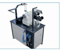
Satin and nylon hanger loop attaching automat with auto cutter and adjustable loop length system.
