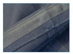
EX 3100 is a semi-automatic sewing machine for mounting the Heading-Tape strip on the trouser hems that have already been closed. The endless roll of Heading-Tape is automatically transferred into the machine mouth. After the sewing the unit cuts the heading-tape and the. The fullness of the tape can be adjusted to suit the material.
