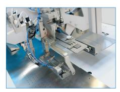
FF 6200-PT is a specially dedicated sewing unit for slanted / Angle Breast Pockets on Men's Jackets ONLY! This PT version is equipped with a matching device for chequered or striped fabrics; with automatic adjustment of the corner knives for the breast welt angles. The unit provides maximum speed and quality compared to manual stiching of the breast pockets on jackets.
