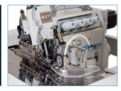
Long seams such as sleeve lining seams, Jacket lining, Jacket side and Jacket back seams are sewn by the sewing unit FX 6300 EXT - IX with a constant high quality.
