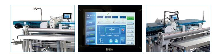
Automatic sewing machine JP 9200-IX is designed for sewing one and two-pointed as well as tapered breast darts on men's jacket and blazers. Easy handling and maintenance
