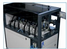
The Automat is used for automatic book-making of up to 8 different washing-care labels from Continuous Rolls of Labels. The automat cuts, optionally folds, collects & puts together 4 to 8 different sizes and lengths of care labels then carries them to the Bartack Sewing head. LB 6310 - IX version is equipped with Ultrasonic Cutting system that can cut all various types of label materials in different dimensions.
