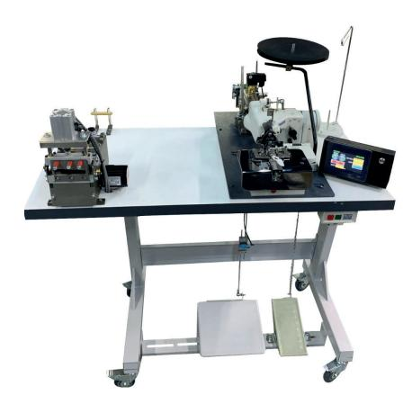
This high-performance blind stitch sewing machine MG 2000 for the standardized and fast fabrication of double-folded belt loops for the classic trousers. The loops come out of the mchine with inserted tapes and are also automatically steam ironed during the process. The machine OPTINALLY comes with an Auto-Cutter system.
