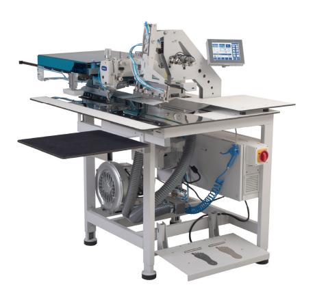
The sewing system OZ 7300-IX is designed for small to medium size trouser production facilities. Besides felling pocket facings on pocket pouches, the left fly piece can be felled and the right fly piece can be felled on and even the right and left pocket facings can be felled at the opening.
