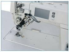
Brother S-7300 A NEXIO is the best Sewing Head with Direct Drive Electronic Transport for making mock pick-stitch (hand stitch pattern on one side and chain stitch on the other side). The sewing feeding system is equipped with step motor, replacing mechanical gears. It has a programmable bottom feed system which prevents pockering on the garment.
