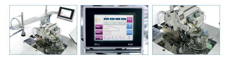
The sewing unit SS 3400 - EX - IX is for automatic serging of trousers without lining as well as skirts and small pieces. The Pegasus EX 5204 head on the automat offers excellent solution for the very fast and rational serging of front and hind trousers parts; skirts and small pieces. The automat has the capability to start the right side leg from the top and left side from the bottom depending on the application.
