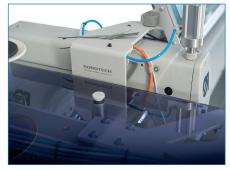
Long seams such as Center-back and sleeve seams are sewn by the sewing unit UK 4100-IX with continuous high quality. The integrated feed technology allows a universal use for different materials.
