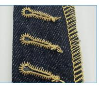
The D-ID 540-S and D-ID 541-A Indexer is for sewing multiple single needle double chainstitch keyhole shaped and round end buttonholes with short tail thread trims on denim fly fronts. The indexer unit ensures buttonholes are sewn automatically one after another at required lengths and pre-set distances from one another. Distance between each buttonhole can be set seperately by the operator on the touch screen display.
