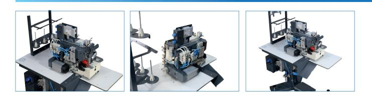
The machine D-WB 540-IX is designed for sewing waistbands of medium heavy to heavy material such as jeans, working pants, Sport pants and Skirts.
